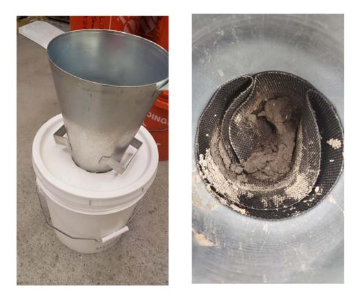
Sample B-6 Geotube Filtration test set-up (left) and 7 day solids (right).
