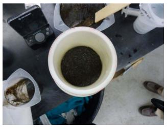
Sample B-6 Rapid Drainage Test filtrate (left) and filter cake (above).
